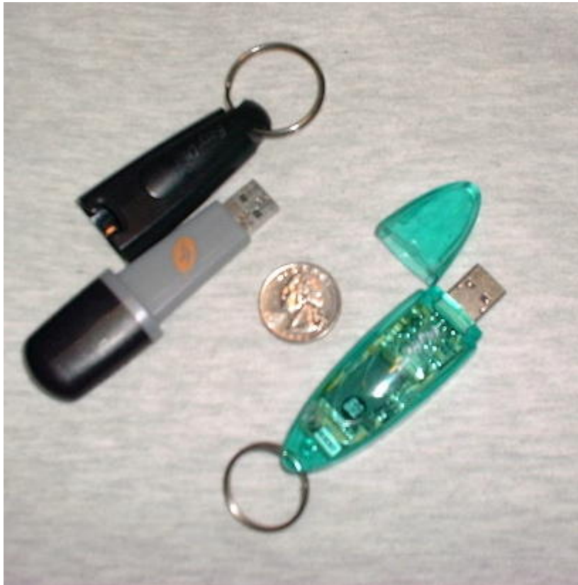
Figure 1. Two USB flash drives. Left: my 32MB Easy Disk. Right: my wife's 128MB Soyo Pen Drive Pro. The Easy Disk's attachment point is on its dustcap, which thus remains on your key chain, belt or wherever, while the business end is in use. Soyo (like most flash drives, unfortunately) flubs this by putting its attachment point on the wrong end.
